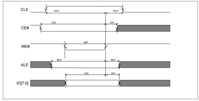
Figure 5. AC Waveforms for Data Input Cycle
