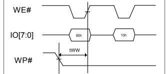
Figure 45-3. Enable Erasing of WP# Signal
