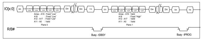
Figure 39. AC waveforms for Two-plane Cache Program (Traditional)
