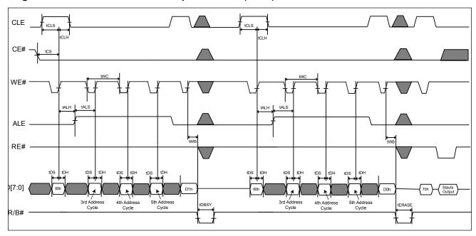
Figure 38. AC waveforms for Two-plane Program (Traditional)
