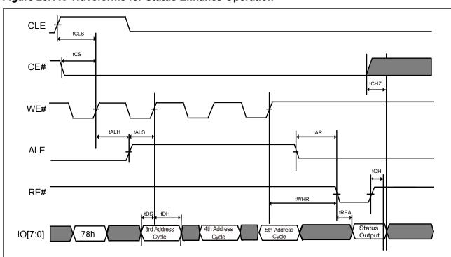
Figure 20. AC Waveforms for Status Enhance Operation
