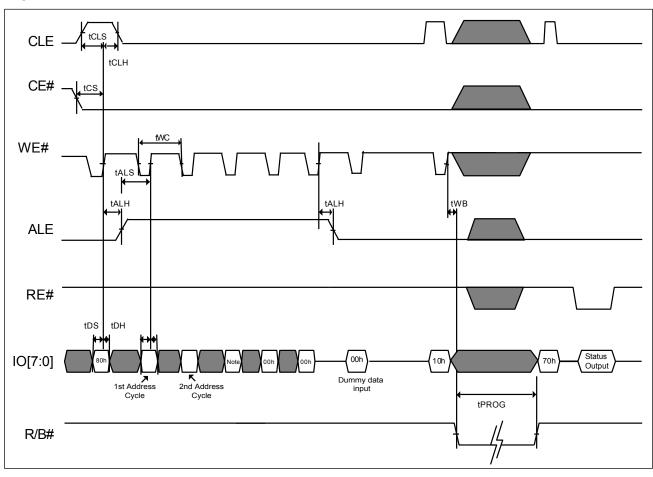
Figure 33. AC Waveforms for OTP Protection Operation
