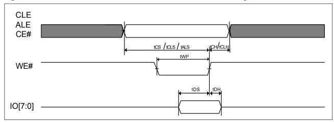
Figure 3. AC Waveforms for Address Input Cycle
