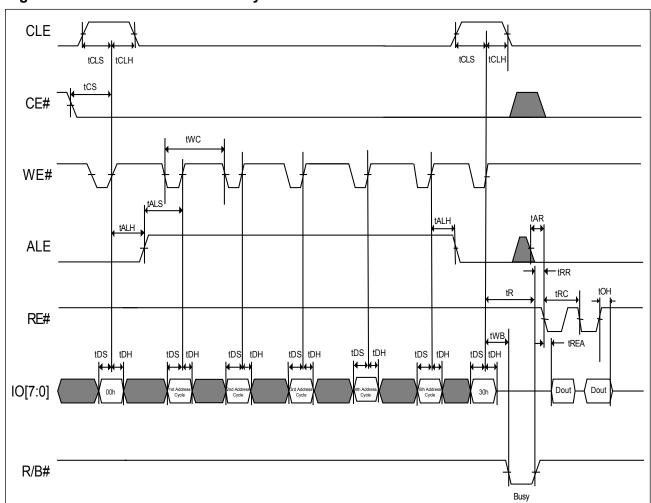
Figure 6. AC Waveforms for Read Cycle
