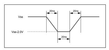
Figure 42. Maximum Positive Overshoot Waveform
