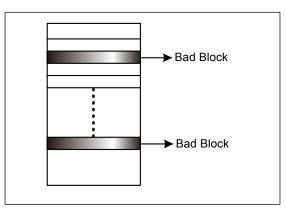
While the device is shipped, the value of all data bytes of the good blocks are FFh. The 1st byte of the 1st and 2nd page in the spare area for bad block will be 00h. The erase operation at the bad blocks is not recommended.
