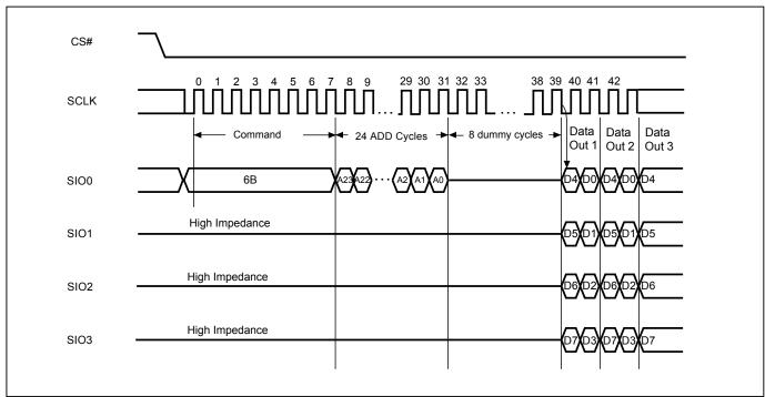
Figure 35. Quad Read Mode Sequence (SPI Mode only)
