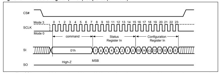
Figure 26. Write Status Register (WRSR) Sequence (SPI Mode)
