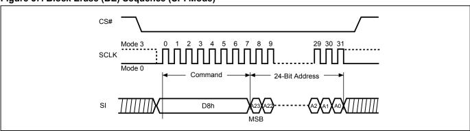
Figure 58. Block Erase (BE) Sequence (QPI Mode)
