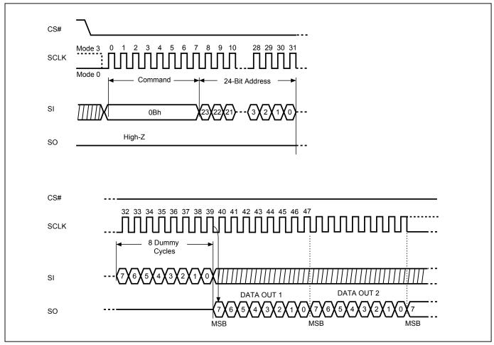
Figure 32. Read at Higher Speed (FAST\_READ) Sequence (QPI Mode)
