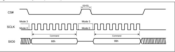
Figure 81. Reset Sequence (QPI mode)
