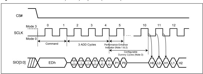
Figure 41. Fast Quad I/O DT Read (4DTRD) Sequence (QPI Mode)
