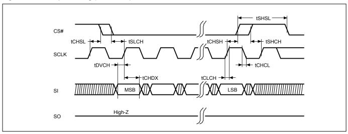
Figure 3. Serial Input Timing (DTR mode)
