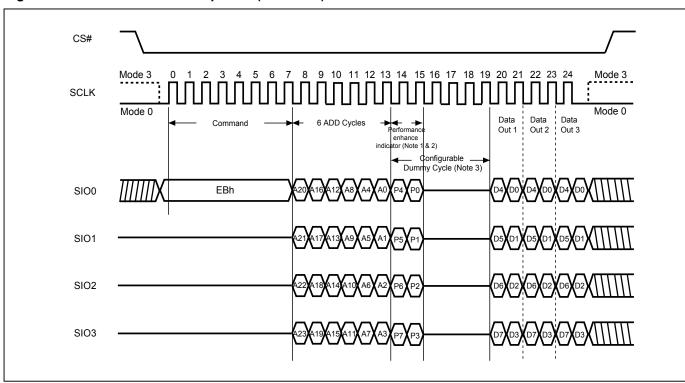
Figure 36. 4 x I/O Read Mode Sequence (SPI Mode)
