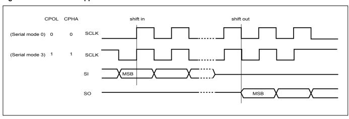
Figure 1. Serial Modes Supported
