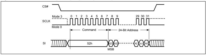
Figure 56. Block Erase 32KB (BE32K) Sequence (QPI Mode)
