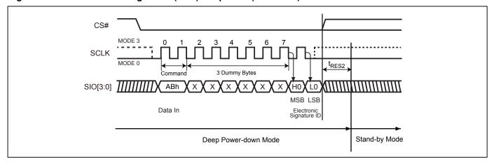
Figure 17. Release from Deep Power-down (RDP) Sequence (SPI Mode)
