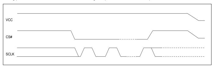
Figure 91. Power-up Timing
