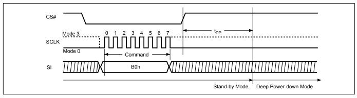
Figure 65. Deep Power-down (DP) Sequence (QPI Mode)
