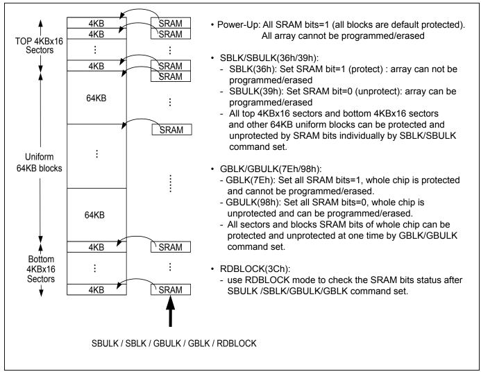
Figure 72. Write Protection Selection (WPSEL) Sequence (Command 68h)
