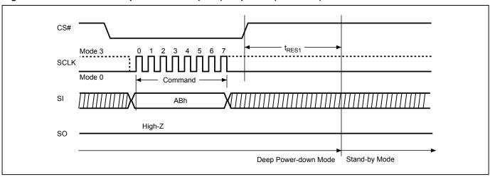
Figure 18. Release from Deep Power-down (RDP) Sequence (QPI Mode)
