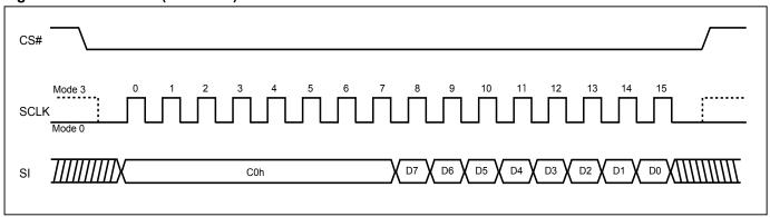
Figure 50. Burst Read (QPI Mode)
