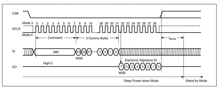
Figure 15. Read Electronic Signature (RES) Sequence (SPI Mode)
