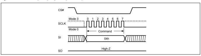
Figure 9. Write Disable (WRDI) Sequence (QPI Mode)
