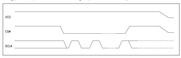
Figure 85. Power-up Timing
