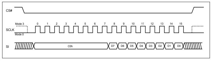
Figure 35. Burst Read (QPI Mode)
