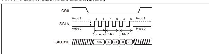
Figure 24. Write Status Register (WRSR) Sequence (QPI Mode)
