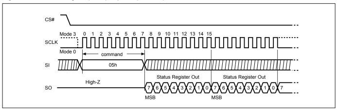
Figure 18. Read Status Register (RDSR) Sequence (QPI Mode)
