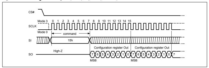
Figure 20. Read Configuration Register (RDCR) Sequence (QPI Mode)
