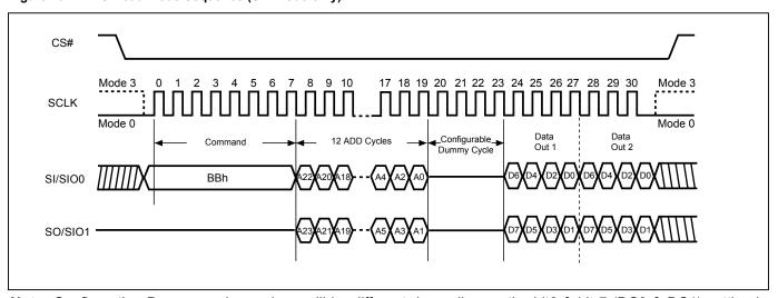
Figure 29. 2 x I/O Read Mode Sequence (SPI Mode only)
