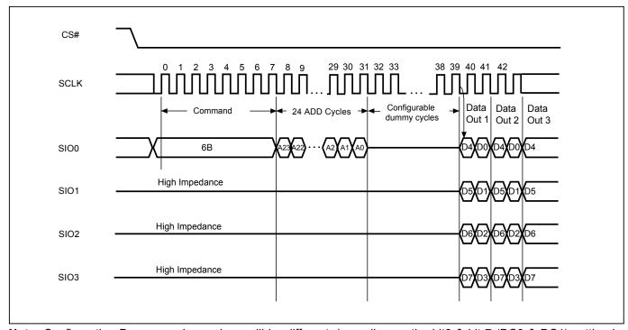
Figure 30. Quad Read Mode Sequence (SPI Mode only)
