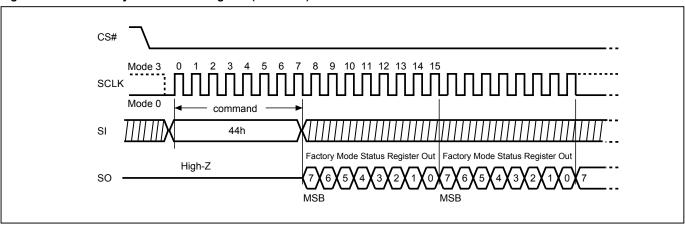
Figure 52. Read Status Register (RDSR) Sequence (QPI Mode)
