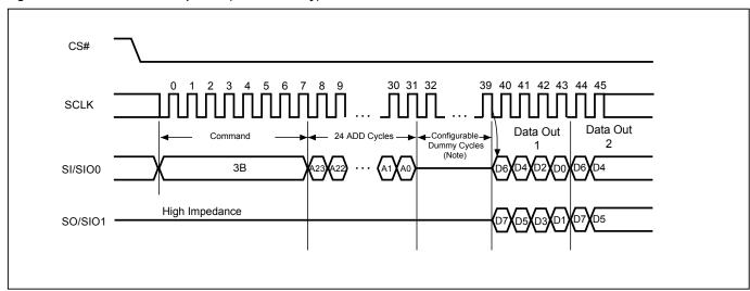
Figure 28. Dual Read Mode Sequence (SPI Mode only)
